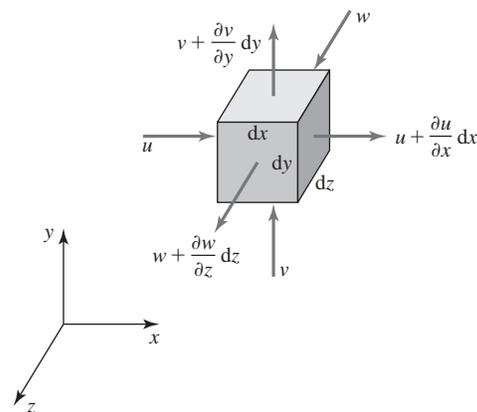
**Figure 8.2** Differential volume element in three-dimensional flow.
